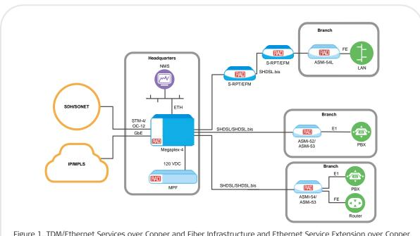
Figure 1. TDM/Ethernet Services over Copper and Fiber Infrastructure and Ethernet Service Extension over Copper Lines
