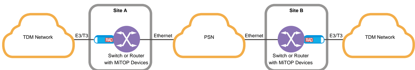
Figure 1. Delivering E3/T3 Services over PSN
