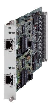
2-channel, high-speed data transmission for the DXC family of modular cross-connects
