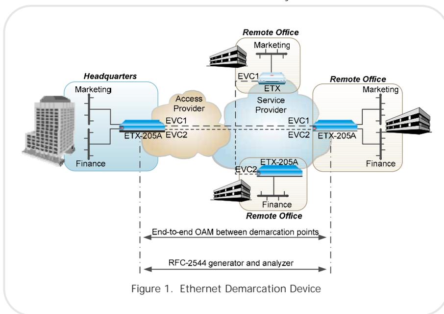
Figure 1. Ethernet Demarcation Device
